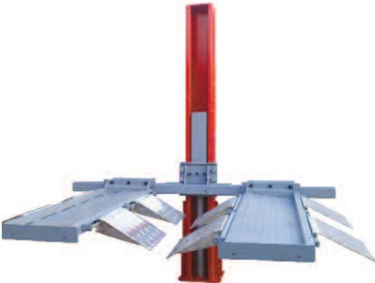
Our Multi-Lift single post is a great lift for picking up ATV's, UTV 's, lawn mowers, golf carts, and just about any small utility vehicle. The single post take up less room in your garage and runs on a 110V power unit. It has adjustable arms to fit a variety of vehicles, it has a removable center deck optional and a capacity of 2,000 lbs. It does need to be anchored to the floor. It stands 9' 4 " high, 8' 7" wide, 7' deep, with a max lifting height of 72".
