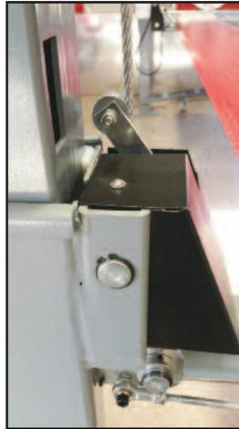
**NEW** secondary slack cable lock system.
