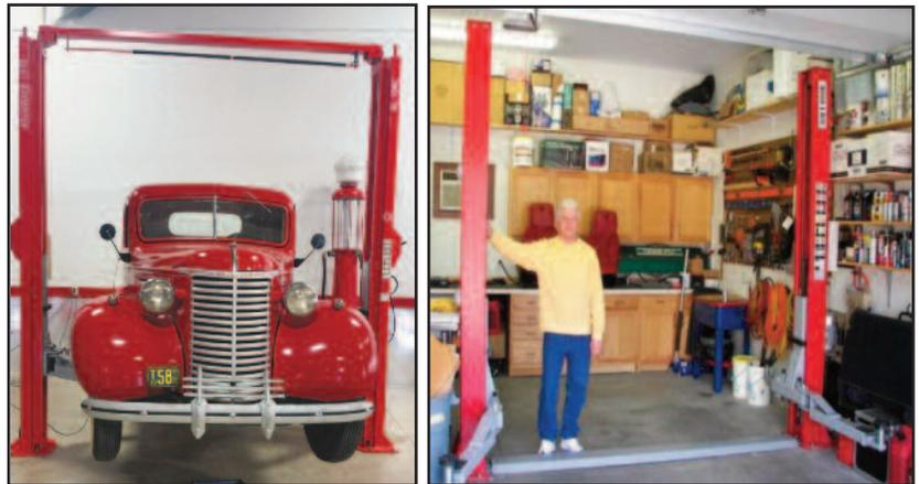
**2 Post Lift.** Looking for a lift to do your brake and tire work? Or remove the body from the frame? We have the lift for you. Two post lifts are seen in almost every service shop across the country. We have two different types to choose from. The Clear Floor with columns 11' 11" tall or the Floor Plate with columns 9' 6" tall with capacities from 9000 lbs. to 11,000 lbs. Adding one of these lifts to your shop or garage will make it much easier to work on your vehicle.
