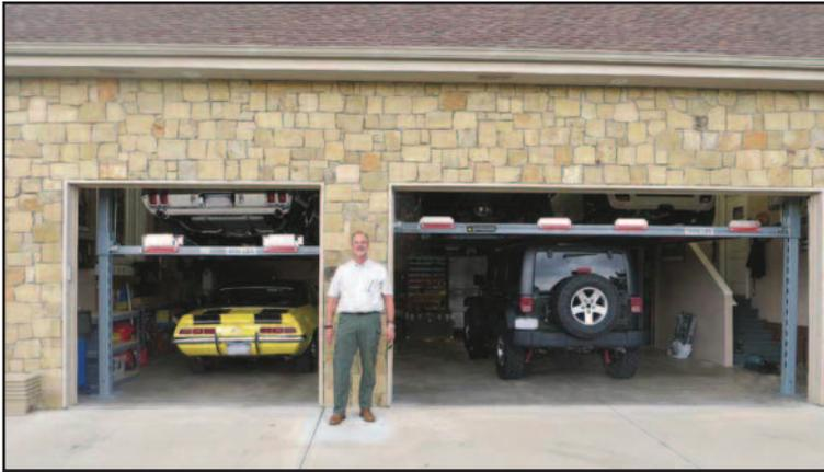
**Side x Side.** The all new Side x Side is a great option for doubling the space of your two-car garage. A span of 16' between the posts gives you ample space to drive two vehicles under your hot rods. With the optional decks it can turn your lift into a mezzanine to store the garage clutter or most anything else. The Side x Side was designed to hold 10,000 lbs. (two 5,000 lb. cars side x side). The cross arms have been pre-arched and re-enforced to prevent sagging.
